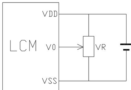
V<sub>DD</sub>-V<sub>0</sub>: LCD Driving voltage
